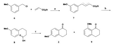
a) Pd(OAc)<sub>2</sub>, Bu<sub>3</sub>N, 100°, 9 h; b) i) H<sub>2</sub>, Pd-C, MeOH, 50 psi, 5 h; ii) 6N, KOH, EtOH,  $\Delta$ , 2 h; c) PPE, CHCl<sub>3</sub>, RT, 7 h.
